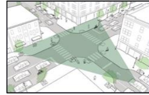
Sight distance improvements
