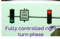
Fully controlled right turn phase
